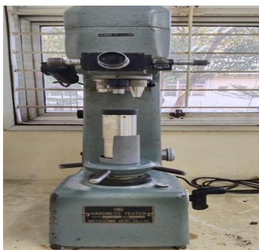
Gambar 5. Micro Vickers Hardness
